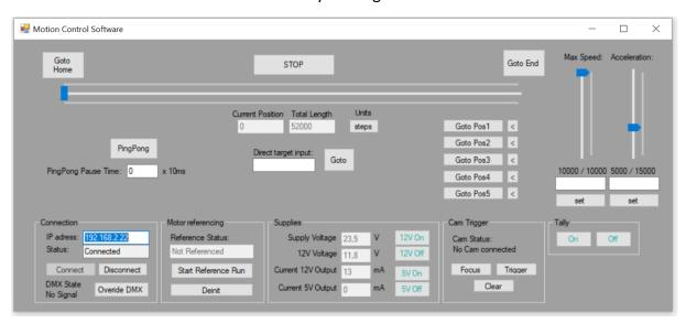
After successful connection, the Status in the connection area shows "Connected" and the slider can be referenced. For this click the "Start Reference Run" button – the slider moves to both ends to learn the length and position of the system.
