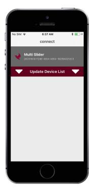
The wireless connection to the Control Unit is established via Bluetooth Low Energy (4.0).
