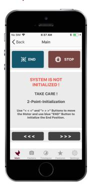
After powering or resetting the Control Unit the system is not initialized. That means the software does not know the position of the slider.
